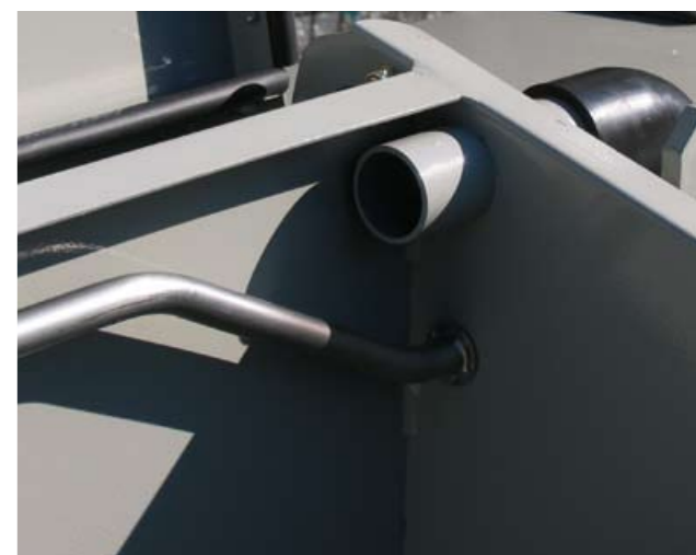
The optional dust extraction is integrated in the mixer grid (SP 11 SM ).
