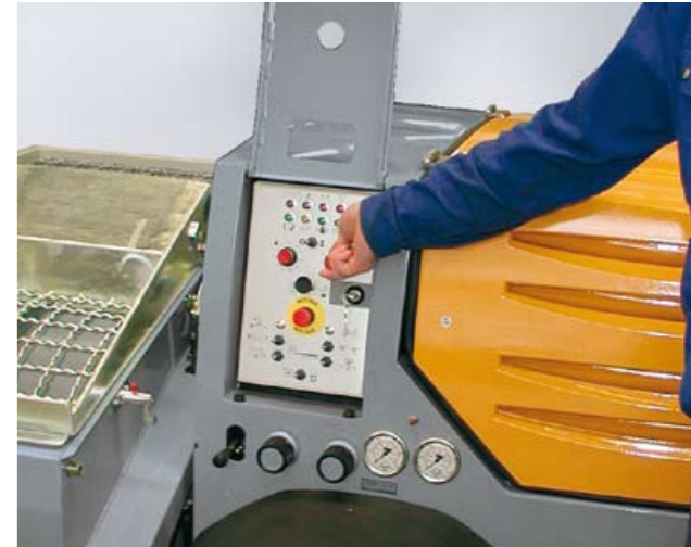
You can control the complete machine from the convenient control panel. A practical flap protects the control panel against dirt and damage.
